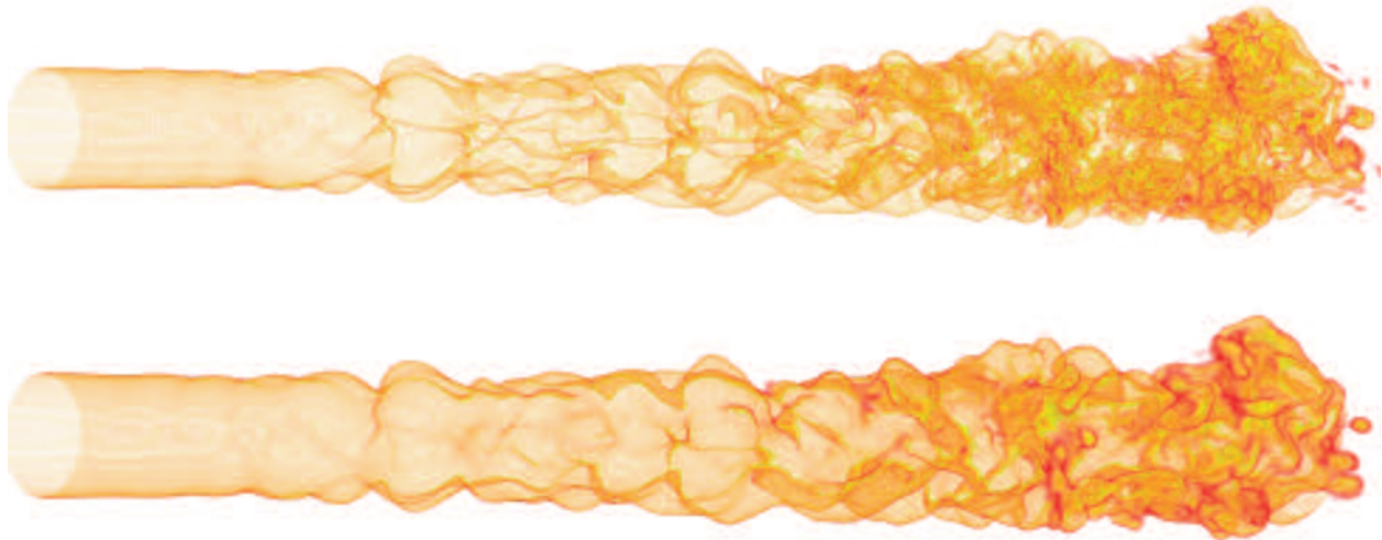
Figure 4. Instantaneous contours of temperature for the DNS (upper image) and hybrid DNS-LES (lower image). In the DNS, the temperature field is fully resolved while in the DNS-LES, only the large-scale temperature is resolved, as it would be in LES. While the temperature fields are very similar, the absence of small-scale mixing is quite noticeable in the lower image. This has the effect of altering the particle nucleation rate by 80%.
