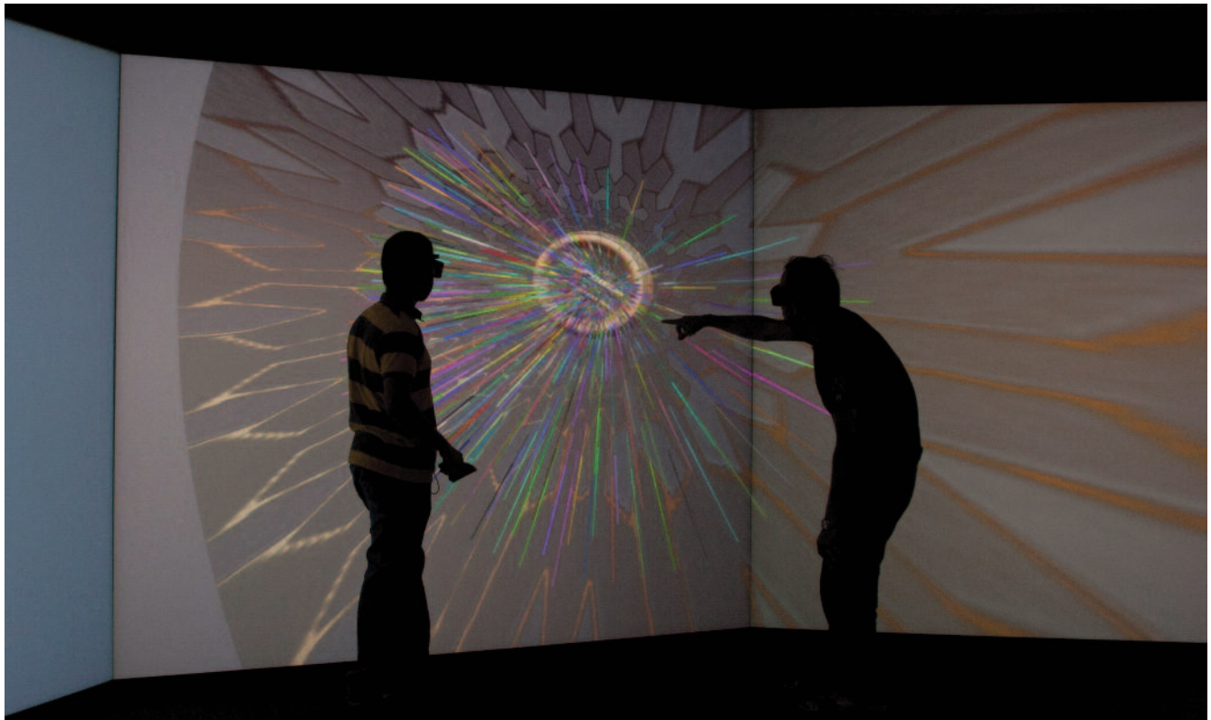
Figure 3. Immersive virtual reality (VR) visualizations provide scientists and engineers with new detailed views of complex anatomical geometries and data. Using the MSI PowerWall, results of a blood flow simulation through an aorta and synthetic heart valve can be explored interactively.
